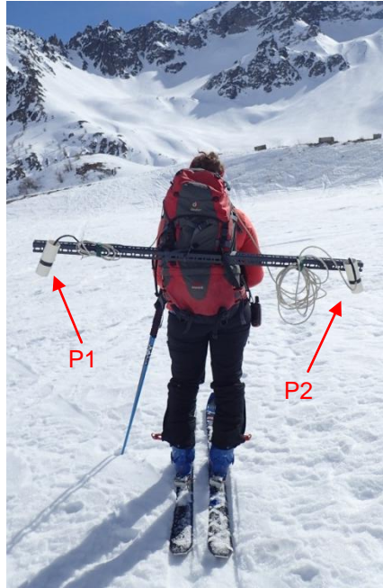
Figure 5: Set up for T_s measurements along the transect at Col du Lautaret. The two IR120 probes were facing the snow surface (P1 and P2 indicated by the red arrows). Measurements were acquired every 20 second on the transect, which corresponds to a distance of 10 m on the transect, on February 26 th , between 08:12 and 12:36 (UTC).
